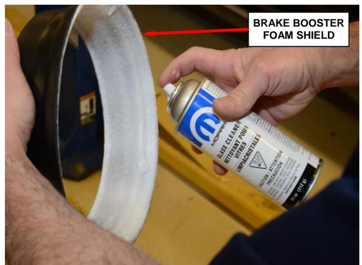
**Figure 11 – Lubricate Brake Booster Foam Shield**
