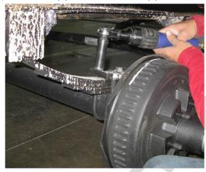
**STEP 1.3** Once the U-bolts are removed; lower the axle enough to insert the 1" spacer block between the leaf spring and axle.
