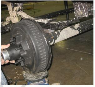
**STEP 1.5** Raise the axle up until the locating pin on the leaf spring aligns with the hole in the top of the 1" spacer. The pin on the 1" spacer block should seat firmly into the hole.
