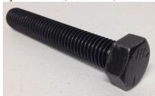
**STEP 4.1** Replace the slide adjustment bolt that is located near the off-doorside (driver's side) front tire. Remove the 4" bolt and replace it with the provided 3" bolt (20X48421A) as provided in the kit.
