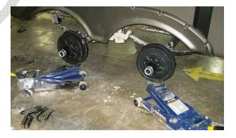
STEP 1.2 With the axles supported, remove the (4) nuts that hold the (2) U-bolts in place. Remove the U-bolts.
