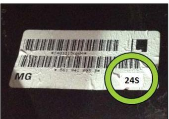
If the Generation Number for both headlights is 24S or higher as shown <circle>, Work Complete, Proceed to Section – Hood Bumper Replacement.
