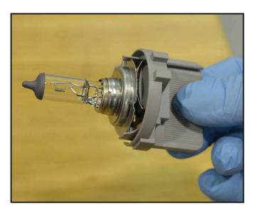
Reinstall the bulb onto the new retainer from kit 561998109 <as shown>.
