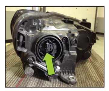
← Remove the low beam headlight bulb retainer <arrow> by turning the retainer to its "keyed" position and sliding outward.
