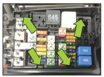
Release the tabs <arrows> while gently lifting the e-box upward out of the housing.
