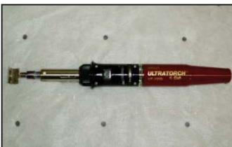
← Set up the UTI-100SI Ultratorch tool or equivalent from the -VAS 1978B- wire harness repair kit <as shown>.
