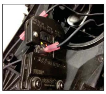
← Crimp the new connector repair harness onto the headlight wiring <as shown> using -VAS 1978/1-2- crimping tool pliers with -VAS 1978/1-1- crimp head in the 0.5mm-1.0mm (red dot) setting.
