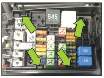
Reinstall the e-box into the housing and press firmly into position to make sure each tab <arrows> is seated fully into place.
