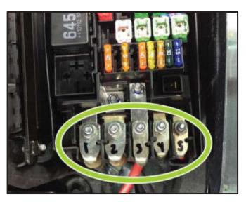
Reinstall each threaded connection accordingly to the E-box <circle> then torque each nut to 9Nm.
