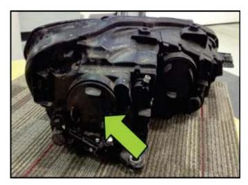
Reinstall protective cover <arrow> and firmly seat into position.
