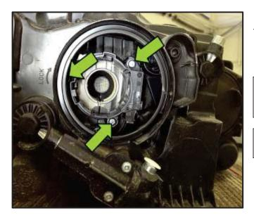
Using a magnetized #1 Phillips screwdriver, remove the three screws <arrows> for the Headlight Socket Retaining Ring and remove ring from headlight housing.
