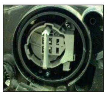
Install bulb retainer assembly into headlight by locking into position as shown <left>.
