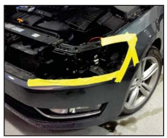
Protect painted surfaces from damage by installing masking tape appropriately as shown.
