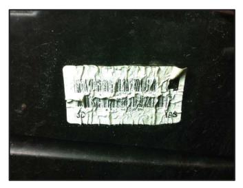
If the label cannot be read as shown <left>, Proceed to Section E - Headlight Assemblies Removed.
