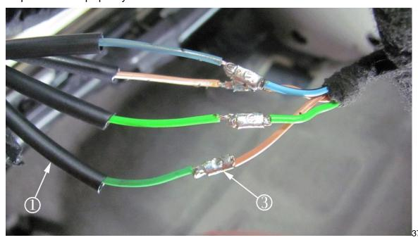
**Warning:** DO NOT use soldering equipment that is battery or electric powered. These types of soldering irons can induce voltage into the circuit, which may cause inflator module deployment and/or damage to electrical components. Use only the EL-28125-5 Ultra Torch or another butane fueled soldering iron when working on SIR circuits.
