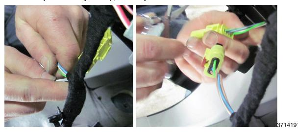
4. Remove 76 mm (3 in) of conduit and tape on both sides of the yellow connector to gain access to the wires.
