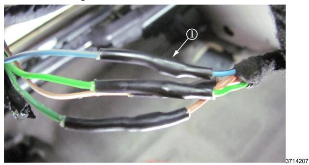
11. Center the heat shrink tube (1) over the splice and use the Ultratorch, part number J-38125-5, or another butane fueled soldering iron, to shrink and seal the heat shrink tube securely over the splice crimp and insulated wires.
