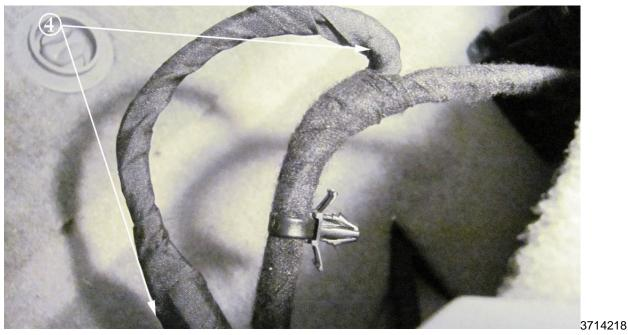
12. Wrap woven polyester electrical tape (PET) or equivalent anti-abrasion tape or electrical tape (4) around the spliced section of the seat and body harness wires.
