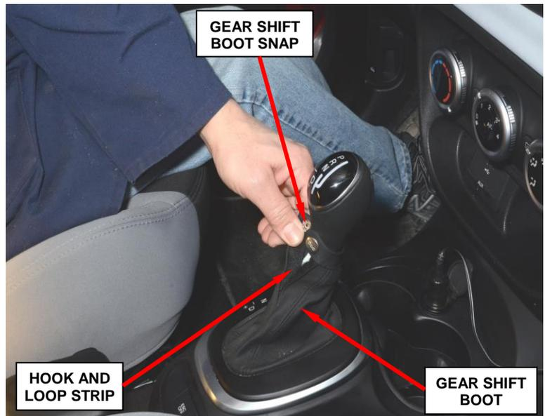
**Figure 1 – Gear Shift Boot**
