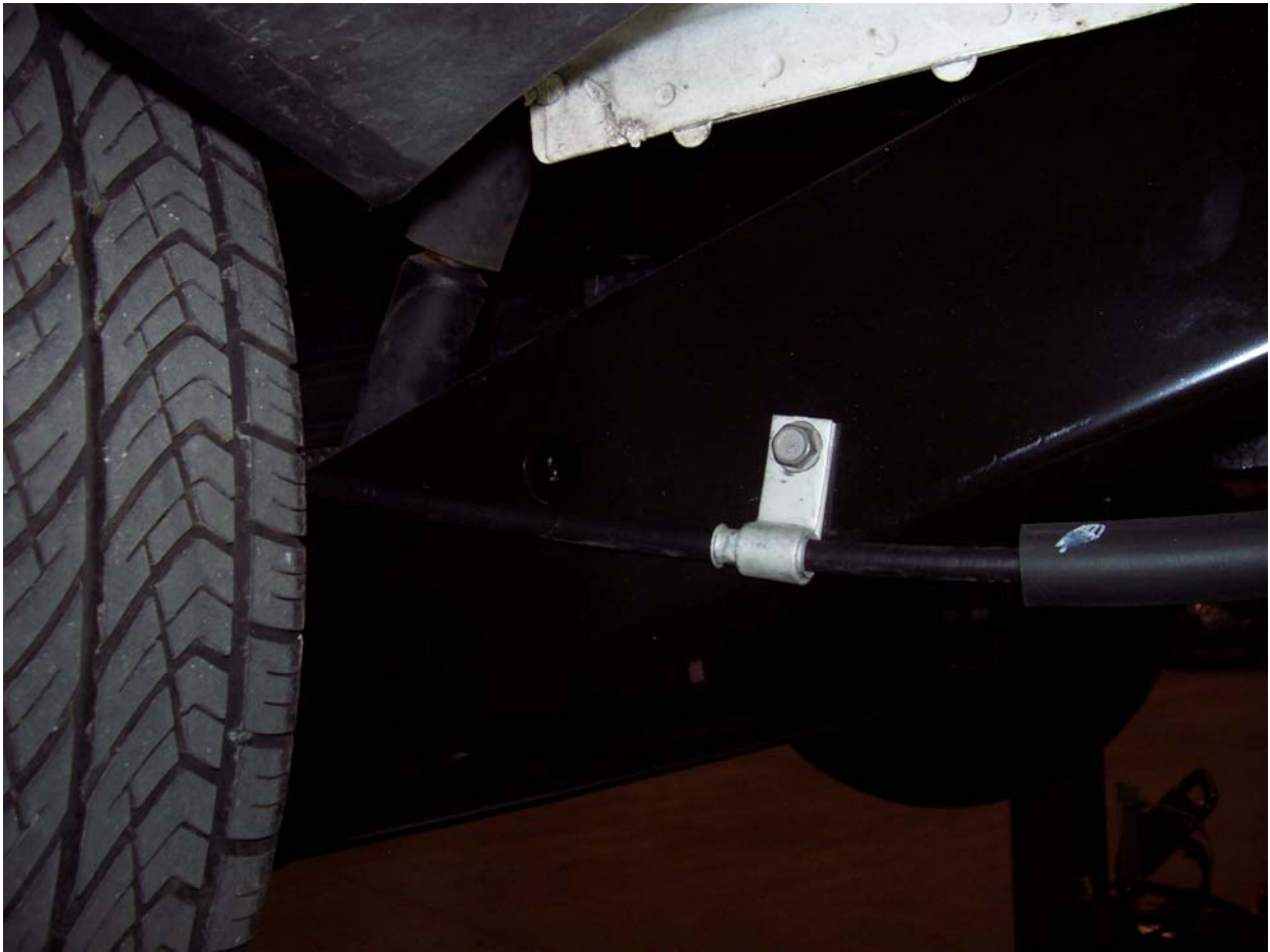
Figure 2: Unscrew parking brake cable bracket from trailing arms
