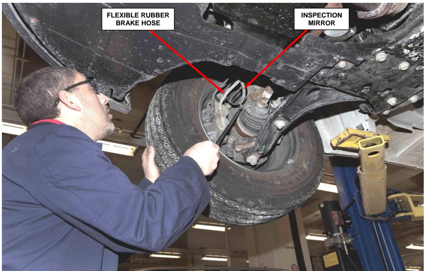
Figure 1 – Inspect Flexible Rubber Brake Hoses at each Brake Caliper (right front wheel shown)
