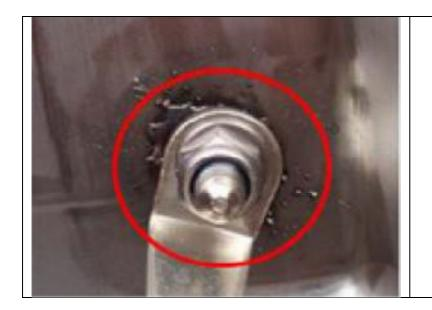
If weld spatter is found or the weld is leaking, <u>do not</u> release the vehicle to the customer. Submit a technical PuMA case and further information will be provided.
