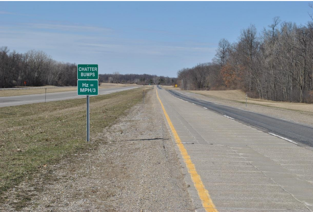
Figure 7a: Chatter Bumps from 55 – 45 MPH – A series of evenly spaced bumps that excite suspension motion. Frequency (cycles per second) = mph /3
