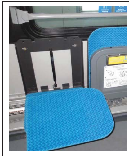
Figure 2 - Seat Backrest Removed from the Frame
