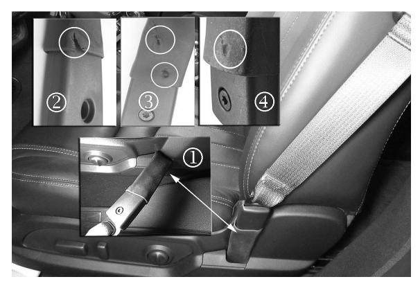
**Note:**With the vehicle door fully open, it will be necessary to pull the safety belt assembly away from the seat until you are able to view the inboard side of the safety belt sleeve (1).
