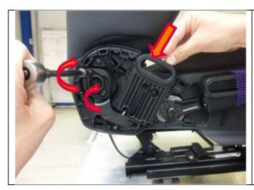
Hold the adjustment lever down so that it touches the rubber stop. While holding the lever down, tighten the two screws to **3 Nm**.
