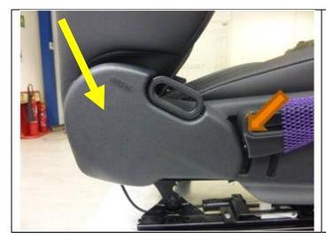
Position the seat backrest in a vertical position (as far forward as possible).
