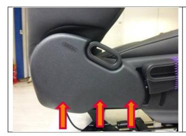
Reinstall the adjustment unit cover.
