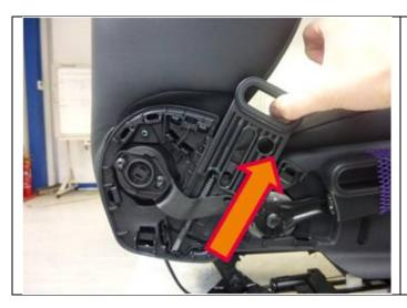
Lift the adjustment lever until the pressure point is reached.
