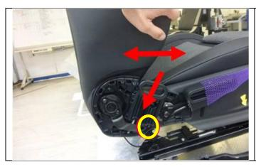
Move the backrest slightly until it engages with the adjuster.
