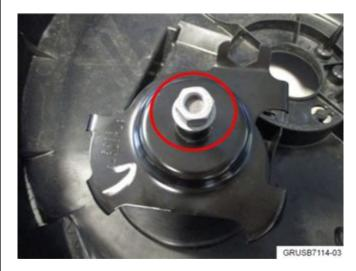
Remove the nut from the bracket holding the compact spare wheel. Fit the new self-locking flange nut (P/N 22 11 6 779 973) and torque to 19 Nm.
