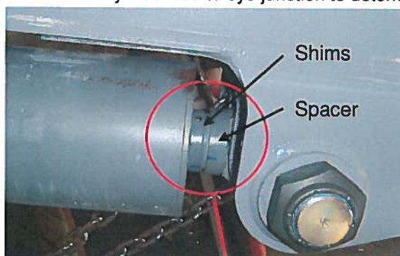
Inspect here on lift cylinder
