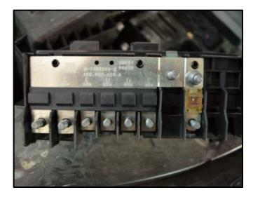
Install the SA fuse panel, 50A fuse, and hex nut onto the new fuse panel assembly as shown <left>.
