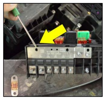
Using a pocket screwdriver, or equivalent, gently pry the SA portion of the fuse panel off the old fuse panel <arrow>.
