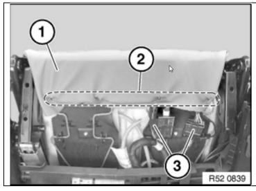
Unhook the seat cover (1) in the area (2). Disconnect the plug connection (3). Remove the seat cover (1) complete with support.
