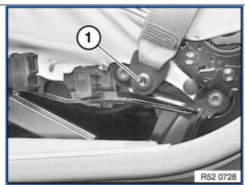
Release the screw (1) for belt mounting.
