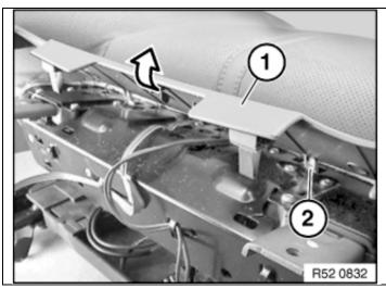
If necessary, unclip the trim (1) towards the top and remove.
