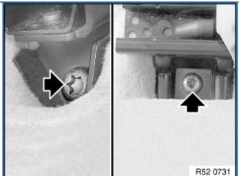
• Release the front screws on the left and right seat rails.
