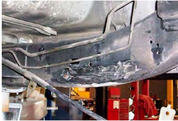
Figure 85 – Frame After Bracket Removal
