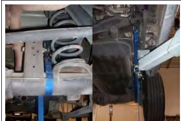
Figure 27 – Ratchet Straps Installed
