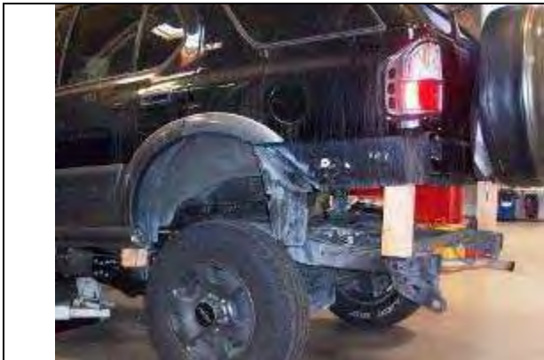
Figure 55 - Wood Block Installed at #5 Body Mount
