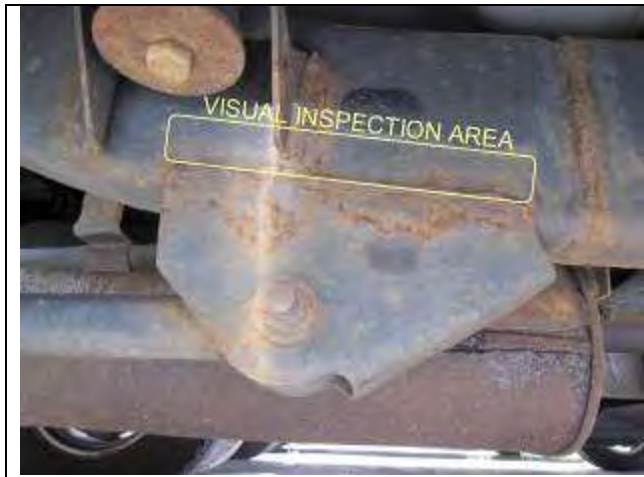
Figure 1 – Visual Inspection Area
