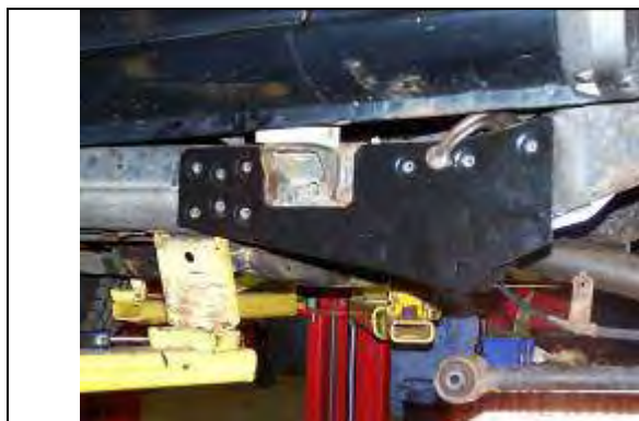
Figure 87 – Type “D” Bracket (temporary installation)
