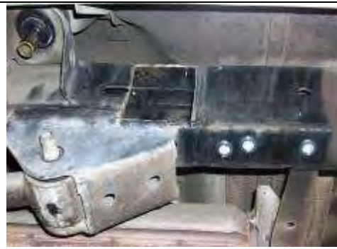
Figure 22 - Passenger Side Pop-nuts Installed
