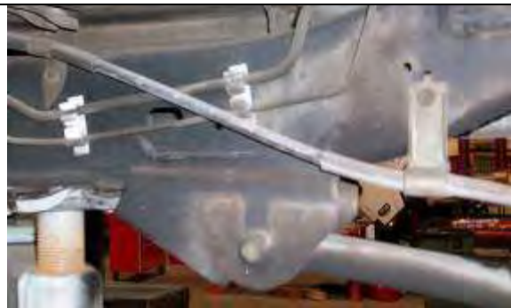
Figure 84 – Passenger Side Bracket Before Removal
