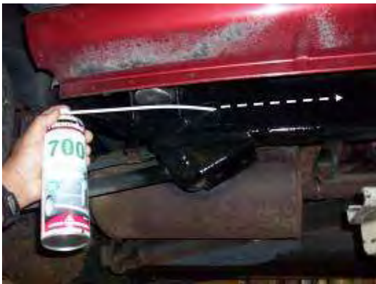
Figure 10 – Frame Hole Toward Front (300 mm)
