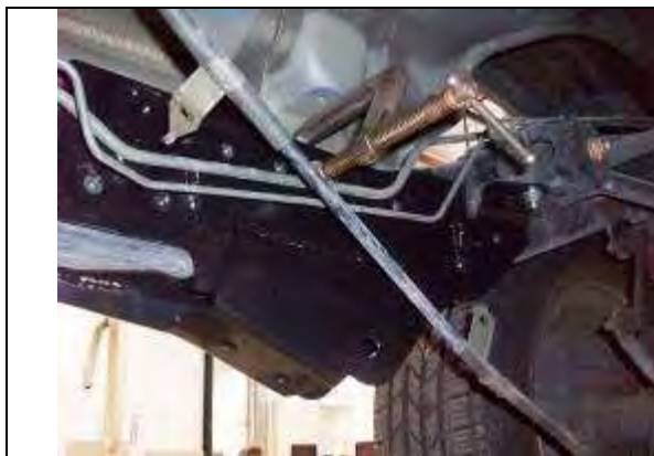
Figure 61 - Type "B" Bracket (temporary installation)
