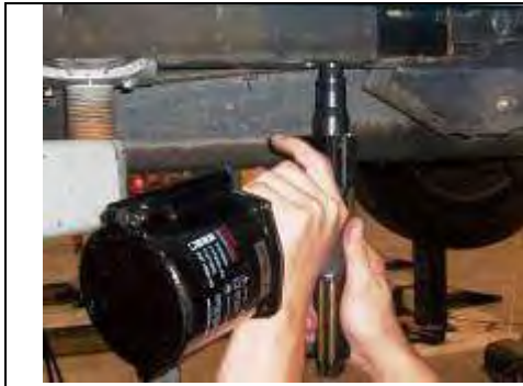
Figure 21 - Pop-nut Installer Ready for Use
