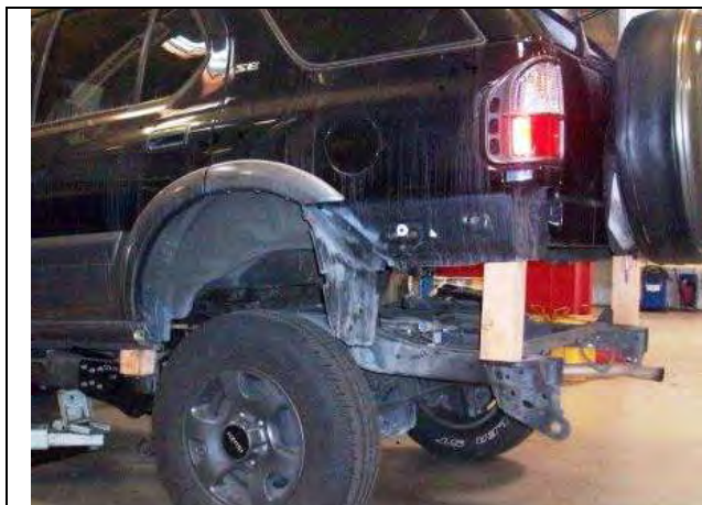
Figure 81 – Wood Blocks Installed at #5 Body Mount
