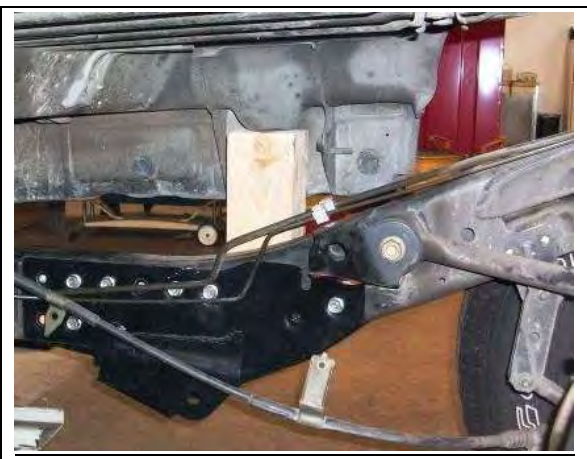
Figure 82 – Wood Block Installed at #3 Body Mount
