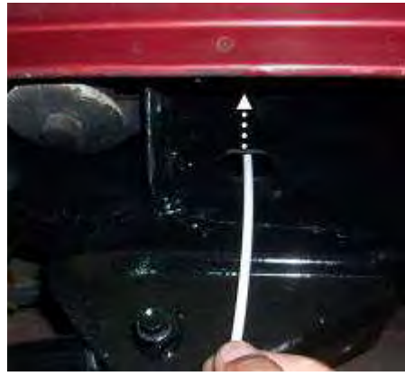
Figure 13 - Frame Hole Up
