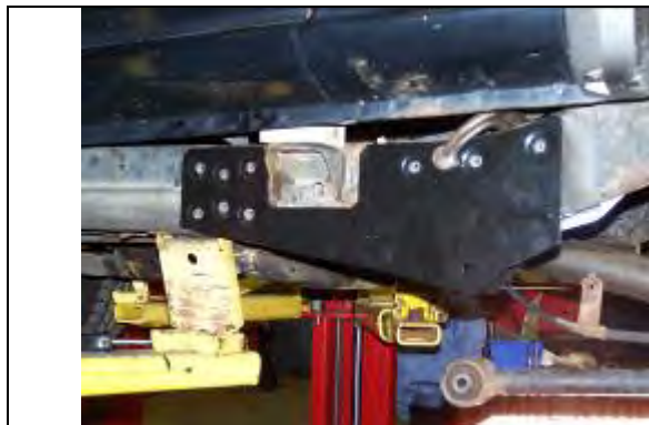
Figure 87 – Type “D” Bracket (temporary installation)
