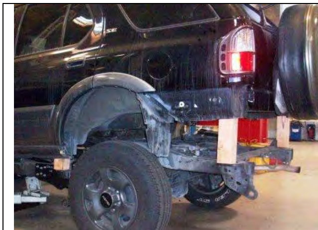
Figure 81 – Wood Blocks Installed at #5 Body Mount
