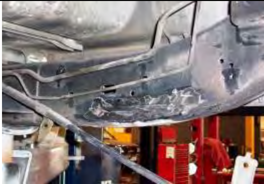
Figure 59 - Frame After Bracket Removal
