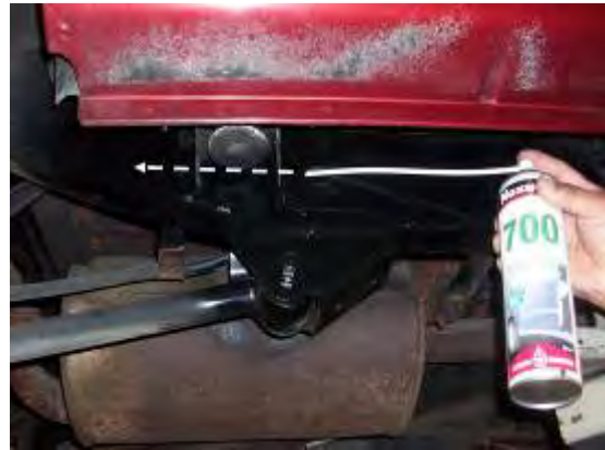
Figure 11 – Frame Hole Toward Rear (300 mm)
