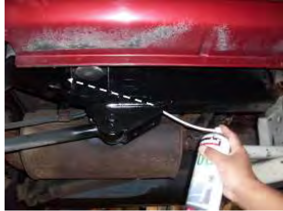
Figure 9 - Nozzle Path (300 mm)
