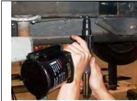
Figure 21 - Pop-nut Installer Ready for Use
