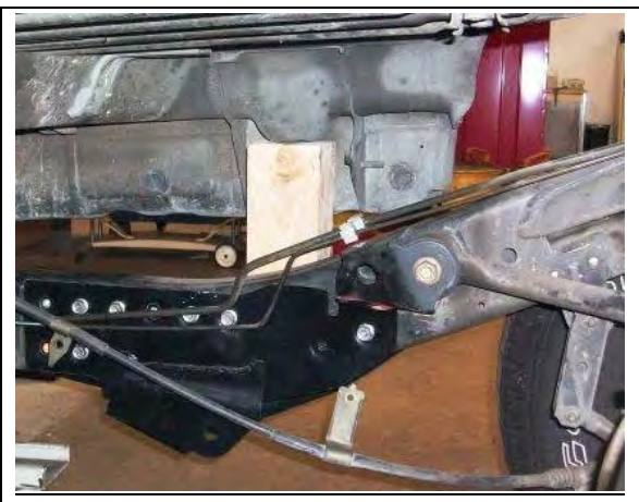
Figure 82 – Wood Block Installed at #3 Body Mount
