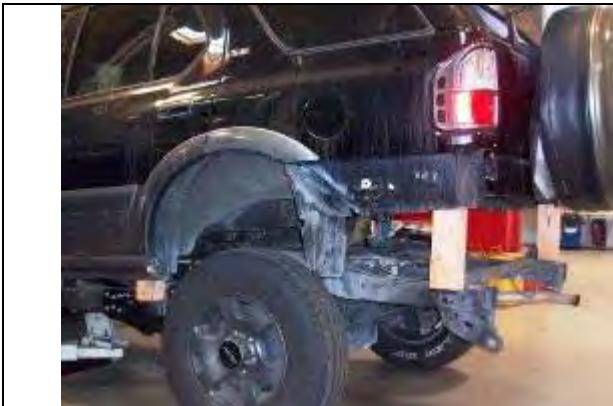
Figure 55 - Wood Block Installed at #5 Body Mount
