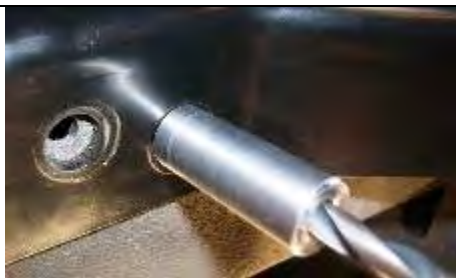
Figure 30 – Drill Guide and Bracket
