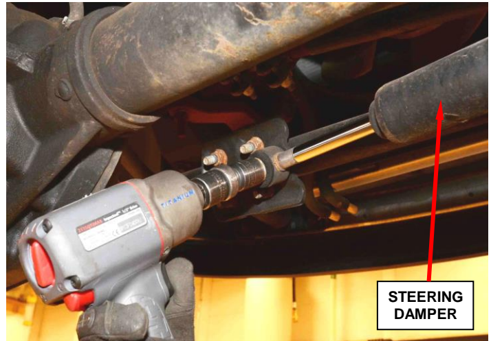
Figure 3 – Steering Damper Nut
