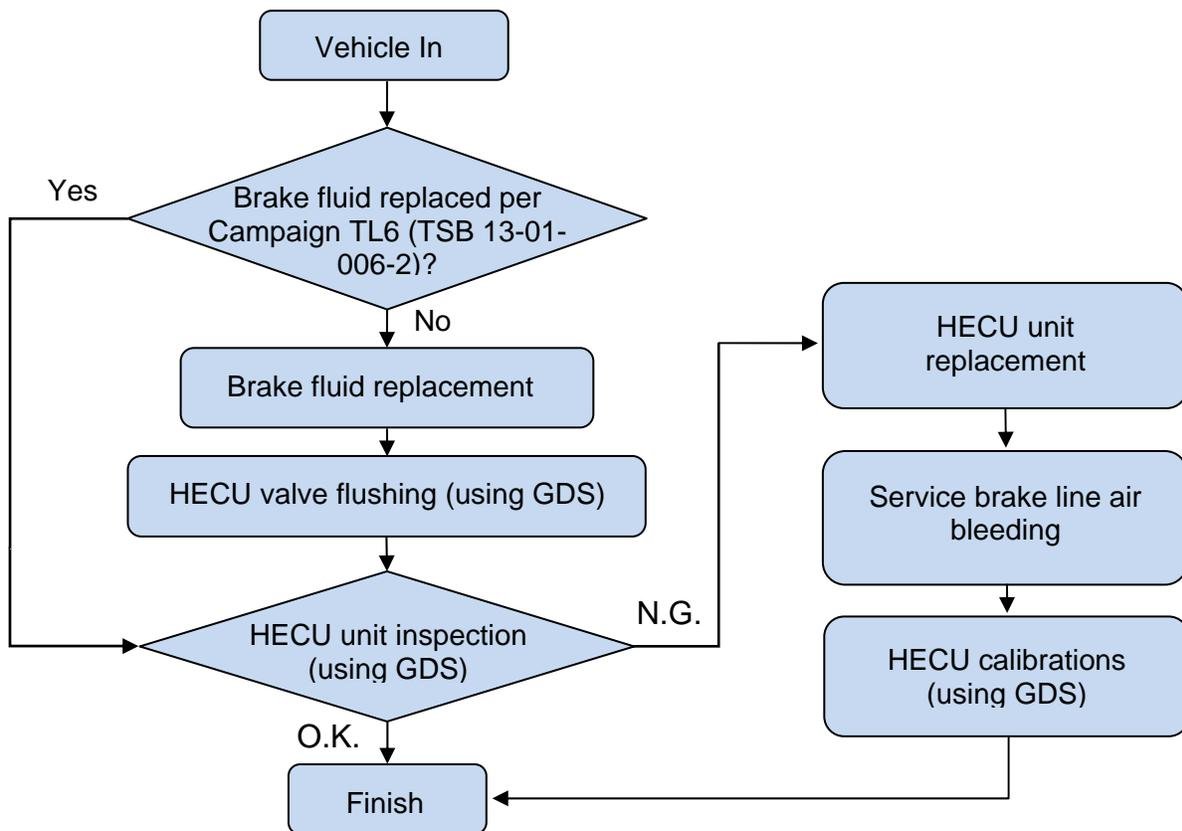
**Service Procedure: Brake Fluid Replacement and Service Brake Line Air Bleeding**
