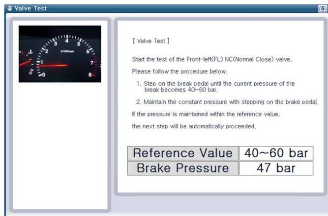
7. While maintaining foot pressure on the brake pedal, check that pedal moves down approximately 30mm (1.18”):
