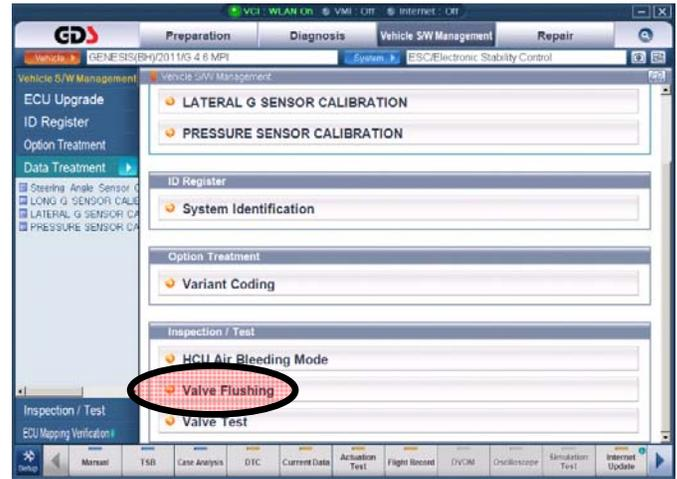
4. As directed by the GDS, press and hold the brake pedal to maintain about 50 bar (725 psi) of brake pressure. Press “NEXT” while holding pressure.
