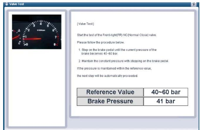
10. After all four valves are tested, the test is complete. Press the “OK” button to finish:
