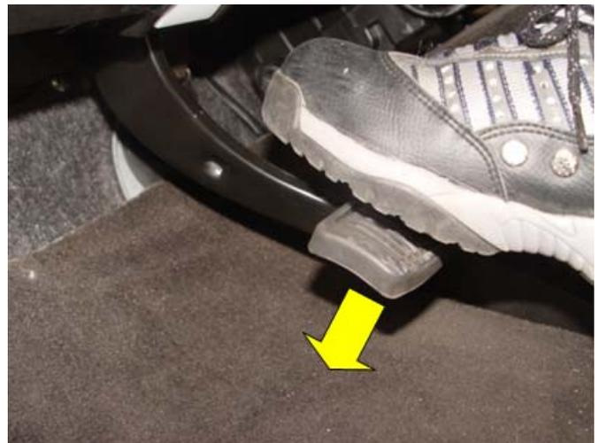
7. Repeat step 6 until the level of brake fluid in the reservoir drops from MAX to MIN.
