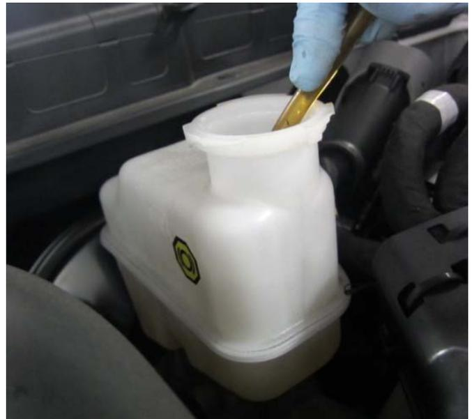
3. Fill the reservoir to the MAX line using DOT4 brake fluid.
