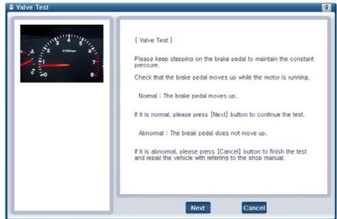
9. The valve test continues with the front right NC (normally closed) valve.
