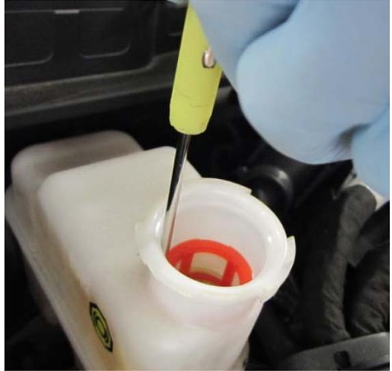
2. Remove as much of the brake fluid as possible using a vacuum pump or similar tool.
