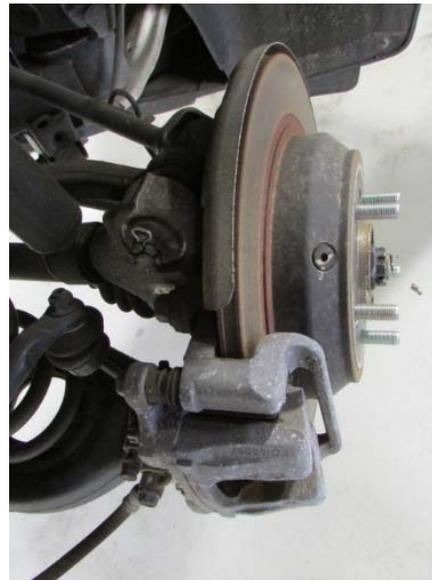
6. Pump the brake pedal 3 times and then hold the pedal down to pressurize the system.
