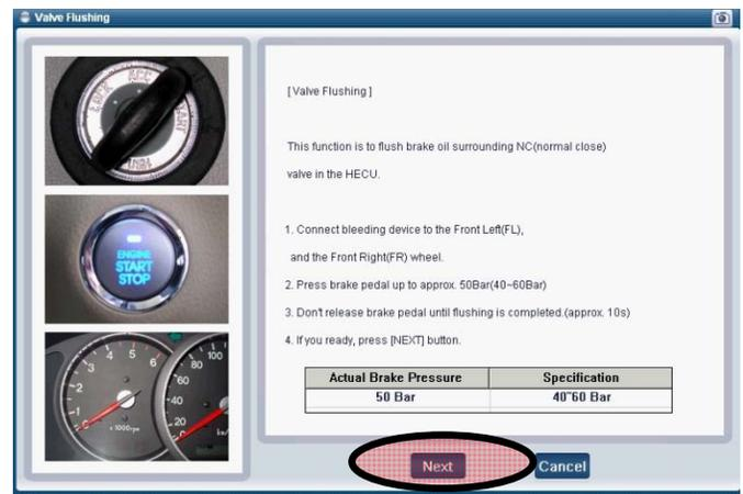
5. The HECU motor will operate and the brake pedal will pulsate for 10 seconds. Maintain holding brake pressure during this time.
