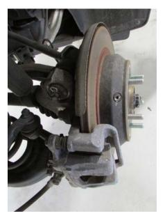
6. Pump the brake pedal 3 times and then hold the pedal down to pressurize the system.
