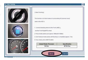
The HECU motor will operate and the brake pedal will pulsate for 10 seconds. Maintain holding brake pressure during this time.
