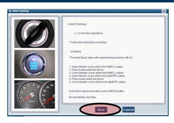
7. Repeat steps 5 and 6 for a total of 10 HECU valve flushing operations. GDS menu screen will count number of iterations.
