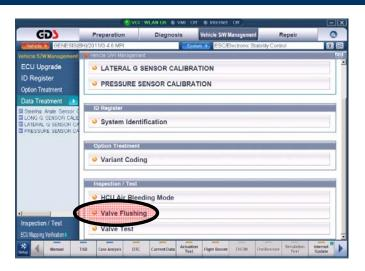
4. As directed by the GDS, press and hold the brake pedal to maintain about 50 bar (725 psi) of brake pressure. Press "NEXT" while holding pressure.
