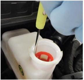
Remove as much of the brake fluid as possible using a vacuum pump or similar tool.
