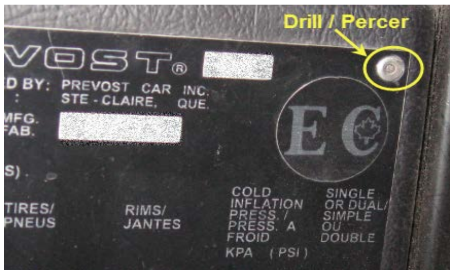
Fig.7 Rivets to be removed (4X).
