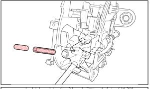
b) Wipe the grease from the pin detent and compression spring.
