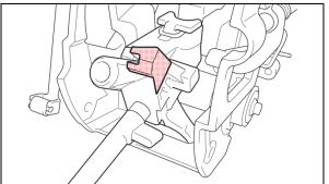
c) Wipe the grease from the highlighted area at the base of the shift lever.
