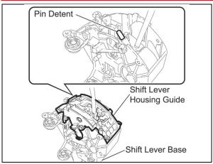
b) Confirm the shift lever in in the N position, then carefully remove the housing from the base.
