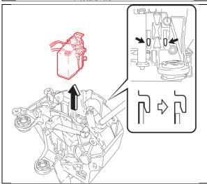
e) Lift up on the solenoid to disengage it from the 2 guides, then completely remove the solenoid.
