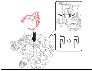
a) Slide the solenoid into place and engage the 2 guides of the solenoid.
