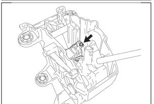
d) Remove the screw at the top of the solenoid.
