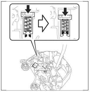
b) Engage the 2 claws to secure the shift lock release link into place.
