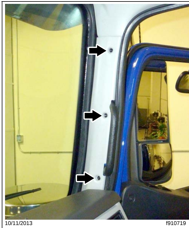
Fig. 3, A-Pillar Cover Screws
