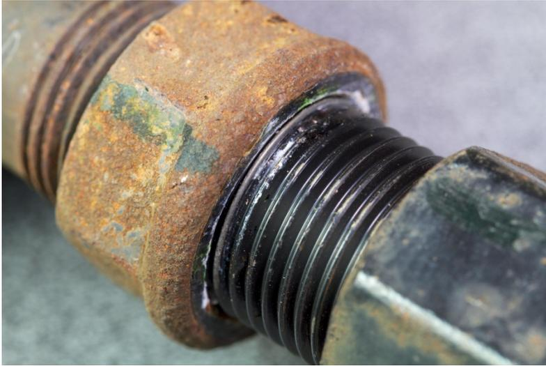
A close-up photograph of a metal suspension arm nut. The nut is heavily corroded with a thick layer of reddish-brown rust. There is a significant amount of white, crystalline residue (likely zinc die-off) covering parts of the nut and the threads of the bolt it is attached to. | <p>Temporarily tighten the arm back to the original condition. Confirm the inspection is performed on both arms then proceed to vehicle alignment.</p> |
