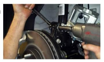
TSB #: 13-01-037 Page 4 of 5 10. Rotate the hub assembly away from the strut and remove axle from the hub. In some cases the axle can be removed with a tug at this point.
