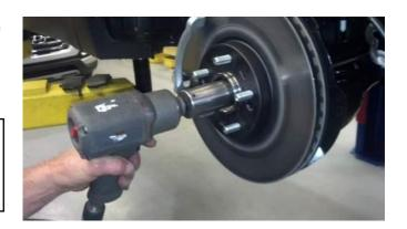
Using a 17mm socket, and 19mm wrench, 9. remove the 2 lower strut bolts, with nuts, and set aside.
