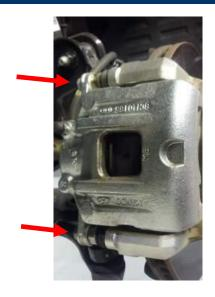
5. Lift caliper upwards and off the brake pads.
