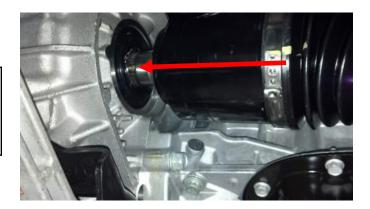
12. With the axle properly installed in the transmission, re-assemble the vehicle by performing the steps in this procedure in reverse order.
