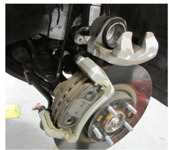
6. Move the caliper out of the way.
