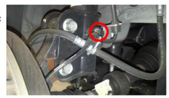
3. Remove the ABS / wheel speed sensor using a 10mm socket, and wrench.
