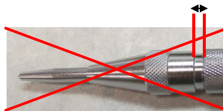
Incorrect Adjustment – Note the gap
