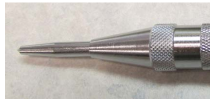
Correct Adjustment – No gap
