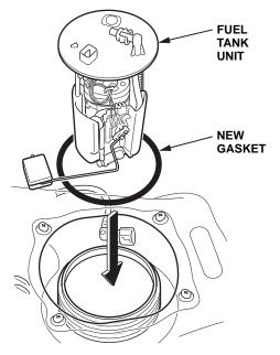
31. Align the marks on the fuel tank and fuel tank unit, then insert the fuel tank unit completely into the fuel tank.
