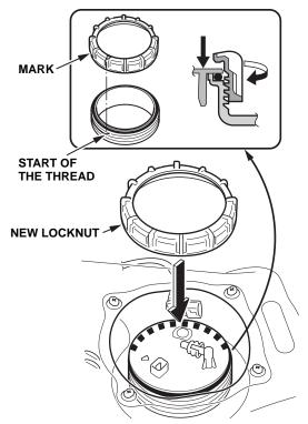
Using the fuel nut wrench, torque the locknut to 100 N•m (74 lb-ft).
