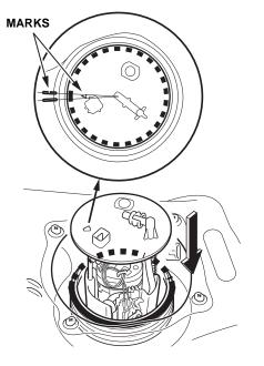
32. Position the new locknut on top of the fuel tank unit, making sure to align the mark on the locknut to the start of the thread. Then, hand-tighten the locknut, holding the unit so it does not move.
