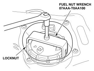
8. Remove the fuel tank unit.
