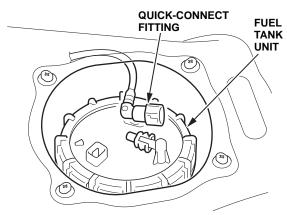
7. Using a fuel nut wrench, loosen the fuel tank unit locknut, then remove it.
