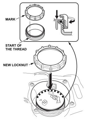
33. Using the fuel nut wrench, torque the locknut to 100 N•m (74 lb-ft).
