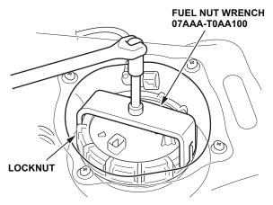
8. Remove the fuel tank unit.
