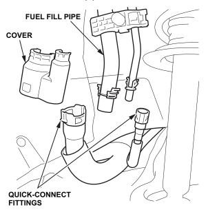
15. Disconnect the quick-connect fittings from the fuel fill pipe and the fuel fill vent hose.
