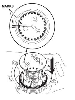
32. Position the new locknut on top of the fuel tank unit, making sure to align the mark on the locknut to the start of the thread. Then, hand-tighten the locknut, holding the unit so it does not move.
