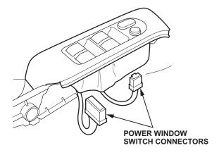
3. Remove the power window master switch cover from the switch panel.
