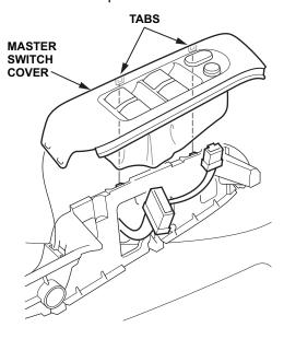
NOTE: Be careful not to break the switch cover tabs when removing the switch cover.
