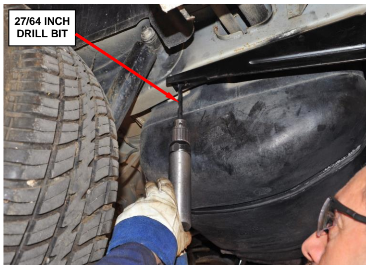
Figure 10 – Drill out Weld Nut(s) Threads
