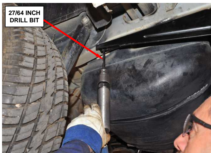
Figure 10 – Drill out Weld Nut(s) Threads
