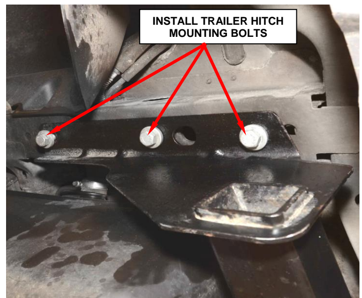
Figure 10 – Install Mounting Bolts (left side shown)
