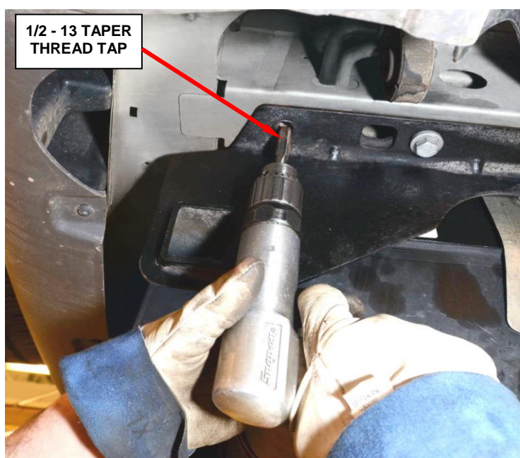
Figure 12 – Tap New Threads into Weld Nut(s)
