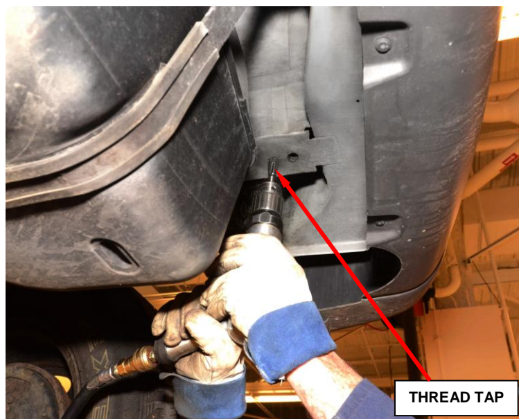
Figure 8 – Chase Threads in Weld Nut with a Tap
