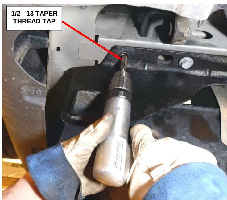
Figure 12 – Tap New Threads into Weld Nut(s)
