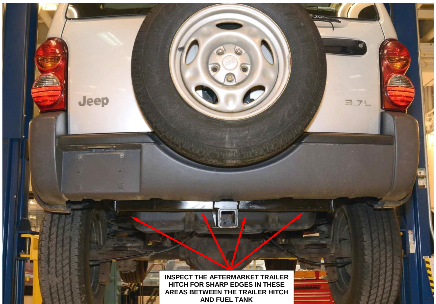
Figure 3 – Inspect Aftermarket Trailer Hitch
