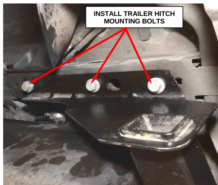
Figure 10 – Install Mounting Bolts (left side shown)
