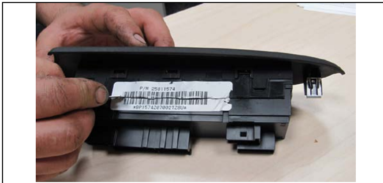
Figure 2 – Using a razor blade or equivalent, cut along the seam of the door module label as shown.
