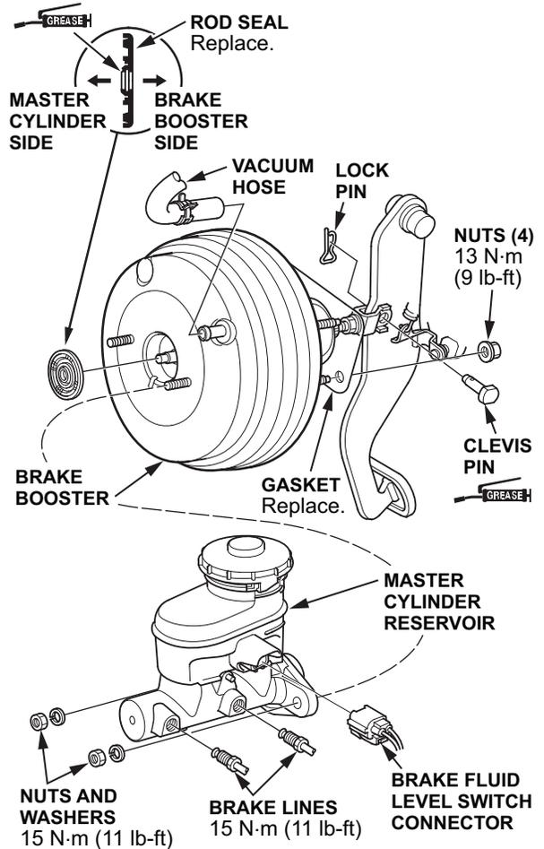
2. Remove the brake fluid from the master cylinder reservoir with a syringe.
