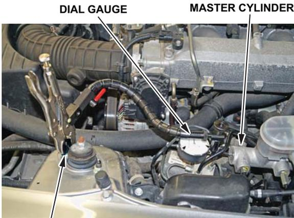
Clamp portion of tool attaches to damper mounting nut.
