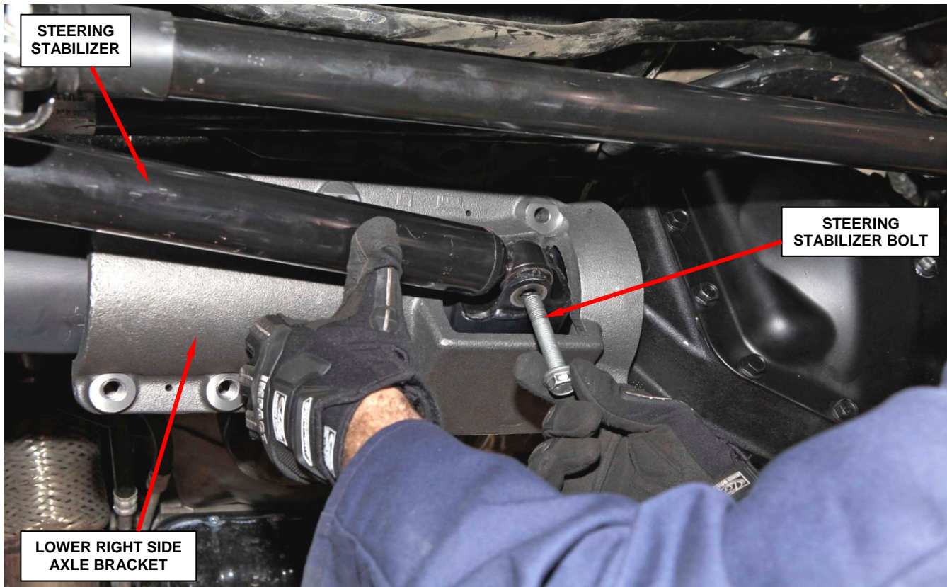
Figure 10 - Install Lower Right Side Axle Bracket
