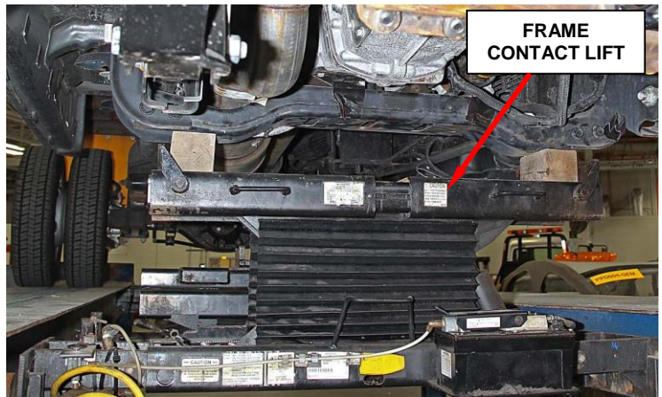
Figure 1 – Raise the Truck Slightly by the Frame
