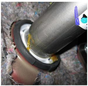
19. Transfer the necessary components from the original to the replacement steering column. Remove the knee protector, ignition steering lock assembly, and dynamic damper from the original steering column. Transfer the dynamic damper and ignition steering lock assembly to the new steering column. Hand tighten the two new shear bolts.
