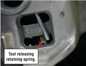
5. **CAREFULLY** lift the airbag module from the steering wheel then turn it over to expose the harness connectors.
