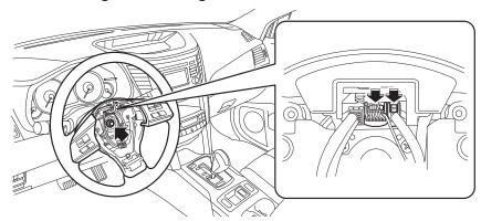
**IMPORTANT:** While removing the steering wheel, and after the steering wheel is removed, make sure the roll connector is not turned from its original arrows aligned (neutral) position as shown below. **NOTE:** Use tape to keep it from turning during and after removal.
