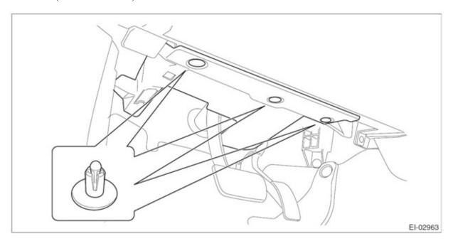
12. After removing the screws, clips and releasing the claws as shown below, remove the instrument panel lower cover as shown below along with disconnecting the wiring harness connectors for the EPB, VDC, etc... switches.
