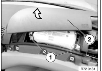
• Undo the screws (1) and place the front passenger's airbag cover (2) on top.
