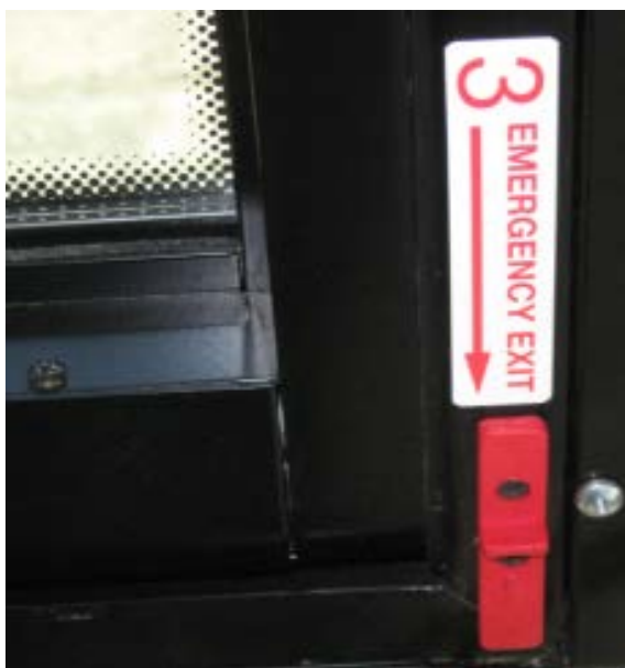
Fig.6b Original Decal To Be Replaced (#790601)
