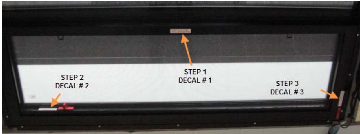
Fig.3 Awning window emergency exit opening sequence.
