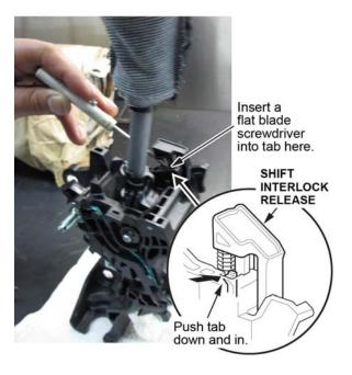
18. Lay the shift lever assembly on its side, and remove the shift interlock release and the spring. NOTE: Make sure you don't lose or damage the spring.
