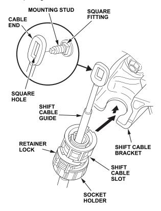
Slide the socket holder onto the shift cable bracket while installing the shift cable end onto the mounting stud by aligning the square hole with the square fitting at the bottom of the stud.
