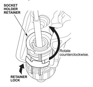
Push the retainer lock in to lock the socket holder retainer in place.
