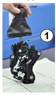
17. Release the shift interlock release by using a pick tool or small flat blade screwdriver (3 mm diameter) to push the tab down and in toward the shift interlock release.
