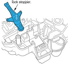
22. Reinstall the shift interlock solenoid by aligning the solenoid plunger joint with the tip of the shift interlock stopper, then push down on the bottom area of the solenoid (side with the printing) until you hear a click.
