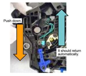
26. Make sure the shift lever moves easily into each gear position. Press the shift interlock release button to move the shift lever out of P.
