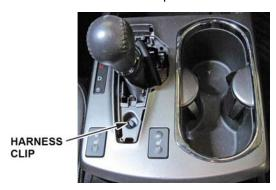
8. Remove the console pocket from the center console panel, and lay it over towards the passenger side.
