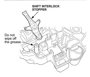
21. Install the new (blue) shift interlock stopper.
