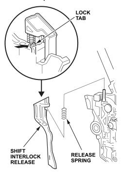
25. Press the shift interlock release button, then release it. Make sure the shift interlock release returns to its original position without sticking or binding.
