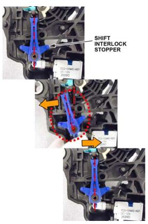
24. Reinstall the release spring and the shift interlock release. Press down on the shift interlock release until you hear a click.
