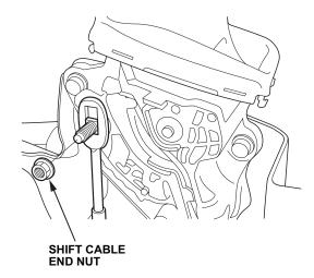
13. Remove the shift cable from the shift cable bracket. First, click on the video below to see how the step is done.
