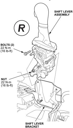
15. Remove the bolt that you inserted earlier to lock the shift lever assembly in the R position.
