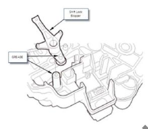
17. Install the new (blue) shift interlock stopper.
