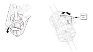
Rotate the upper half (above the retainer lock) of the socket holder retainer counterclockwise until it stops turning.
