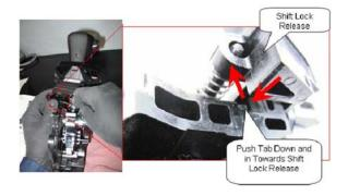
14. After unlocking the tab, lay the shift lever assembly on its side, and remove the shift interlock release and the spring.
