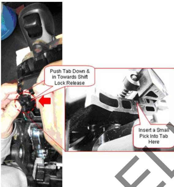
14. After unlocking the tab, lay the shift lever assembly on its side, and remove the shift interlock release and the spring.
