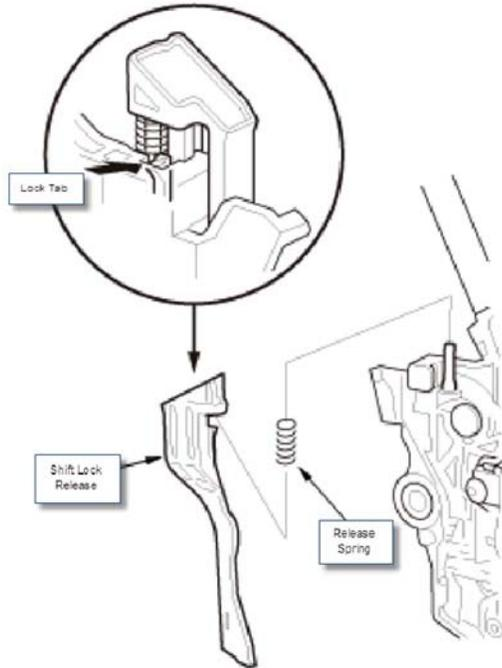
21. Press the shift interlock release button down, then release it. Check that the shift interlock release returns to its original position without sticking or binding.
