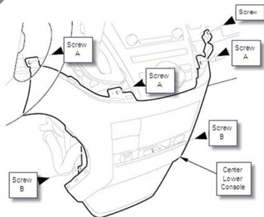
6. Pull the console out far enough to detach the clips, then disconnect the temperature sensor connector and the air hose.
