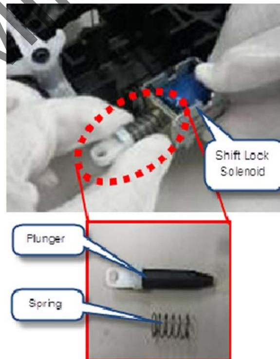
16. Remove the white shift interlock stopper from the shift lever assembly.
