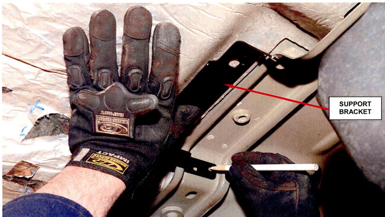
Figure 9 – Mark Hole Locations Using Support Bracket as a Template
