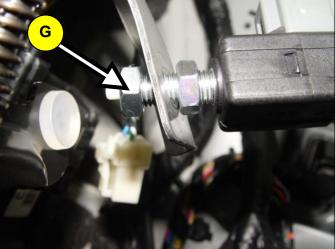
5. Remove the lower mounting nut (G) of the current stop lamp switch.
