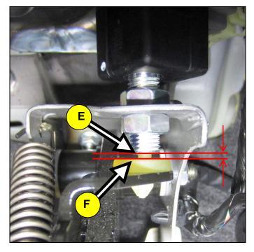
6. Tighten the upper and lower mounting nuts.
