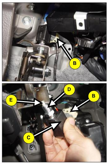
If the stop lamp switch does not operate normally, use the alternative part as shown in the table below.
