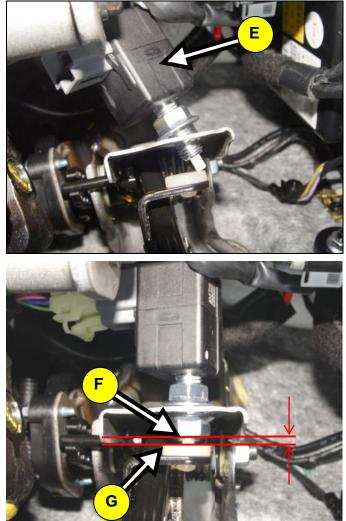
5. Without the brake pedal applied, adjust the gap between the end of the metal threaded housing of the stop lamp switch (F) and the stop lamp switch stopper (G).
