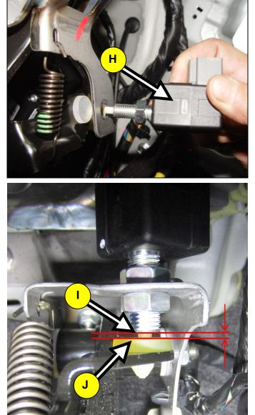
7. Without the brake pedal applied, adjust the gap between the end of the metal threaded housing of the stop lamp switch (I) and the stop lamp switch stopper (J).
