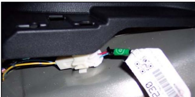
6. Ensure that the fuel sending unit harness is properly connected to the sub-sending unit. If not connected, connect it.
