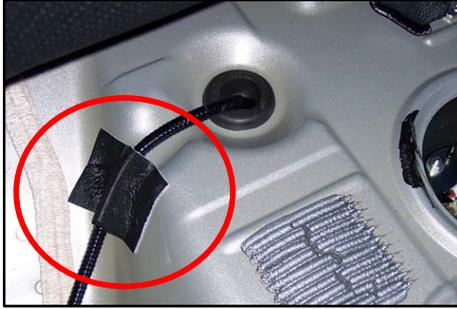
5. Remove the electrical tape and reconnect the negative (-) terminal of the 12V battery.
