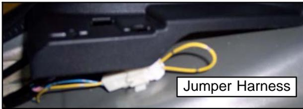
3. Remove the body plug where the fuel sending unit harness is to be installed.
