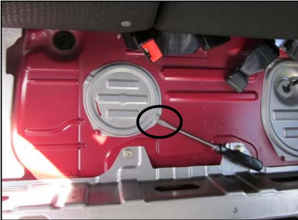
4. On the right hand side of the rear seat area, check for the presence of the fuel sending unit harness. If present, continue to step 5. **If absent, proceed to the Replacement Procedure section.**
