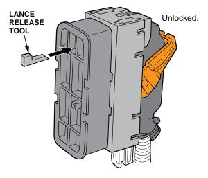
17. Remove the lance release tool, then remove the lance release housing.
