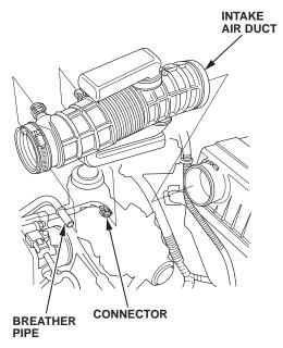
3. Disconnect the VSA control unit 47P connector.
