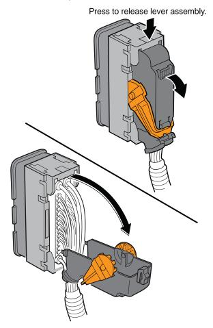
Remove the No. 35 pink wire from the connector while pushing up on the lance release housing.
