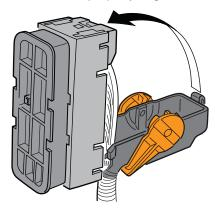
11. Rotate the lever to the unlocked position. The lance release housing also moves into the unlocked position.
