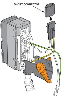
14. Lay out the subharness as shown, then install the lever assembly.
