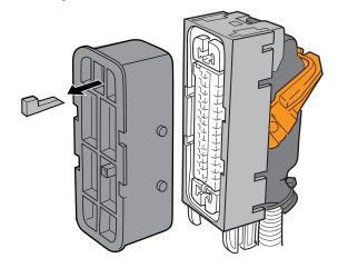
18. Inspect the terminal lock to make sure it is in the locked position.
