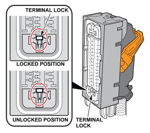
19. Reconnect the 47P connector to the VSA modulator by making sure it is properly aligned, then rotating the lever to the lock position.
