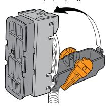
Rotate the lever to the unlocked position. The lance release housing also moves into the unlocked position.
