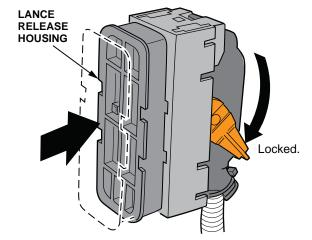
6. Use a small screwdriver to unlock and remove the lever assembly from the 47P connector.
