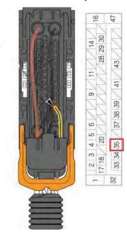
9. Insert the cavity plug remover into the hole in the lance release housing as shown, and push out the plug from the No. 22 cavity.
