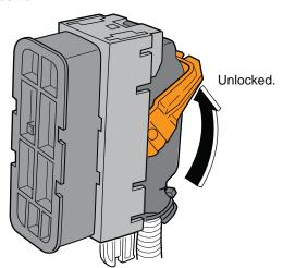
12. Using a small screwdriver, unlock and remove the lever assembly from the 47P connector.
