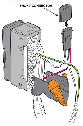
15. Lay out the subharness as shown, then install the lever assembly.
