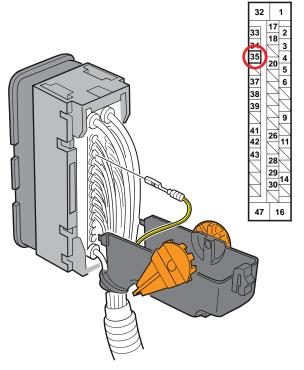
8. Insert the cavity plug remover into the hole in the lance release housing as shown, and push out the plug from the No. 22 cavity.
