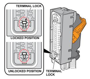
18. Reconnect the 47P connector to the VSA modulator by making sure it is properly aligned, then rotating the lever to the lock position.
