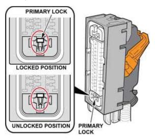
18. Reconnect the 47P connector to the VSA modulator-control unit by making sure it is properly aligned, then moving the lock to the locked position.
