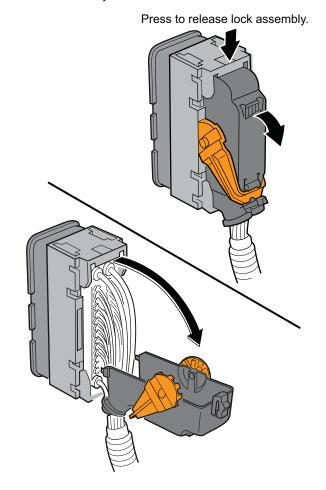
7. Remove the No. 35 yellow/black wire terminal from the connector while pushing up on the lance release housing.
