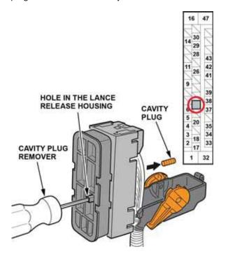
Tuck the loose terminal and wire into the housing, then install the lock assembly onto the 47P connector as shown.
