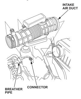
Disconnect the VSA modulator-control unit 47P connector.
