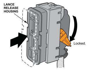
6. Use a small screwdriver to unlock and remove the lock assembly from the 47P connector.
