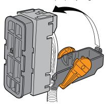
10. Press the lock release tab, then move the lock to the unlocked position. The lance release housing also moves into the unlocked position.
