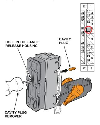
Tuck the loose terminal and wire into the housing, then install the lock assembly onto the 47P connector as shown.
