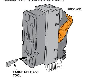
16. Remove the lance release tool, then remove the lance release housing.
