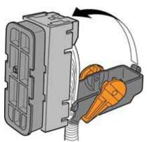
11. Press the lock release tab, then move the lock to the unlocked position. The lance release housing also moves into the unlocked position.
