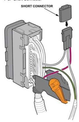
15. Lay out the subharness as shown, then install the lock assembly.
