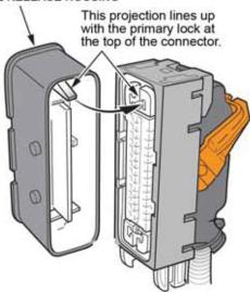
6. Move the lock to the locked position. The lance release housing is fully drawn into the connector and clicks into place.
