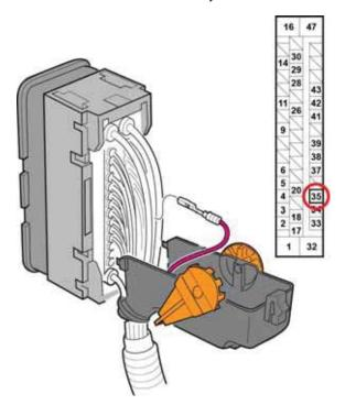
9. Insert the cavity plug remover into the hole in the lance release housing as shown, and push out the plug from the No. 22 cavity.
