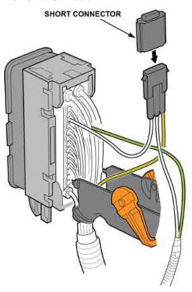
14. Lay out the subharness as shown, then install the lock assembly.
