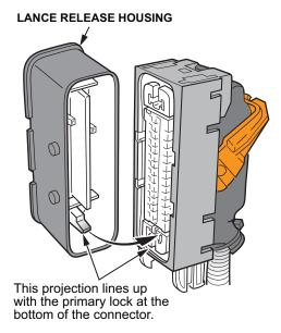
5. Move the lock to the locked position. The lance release housing is fully drawn into the connector and clicks into place.
