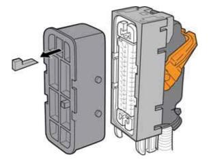
18. Inspect the primary lock to make sure it is in the locked position.
