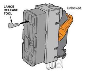
17. Remove the lance release tool, then remove the lance release housing.
