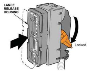
7. Use a small screwdriver to unlock and remove the lock assembly from the 47P connector.
