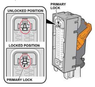
19. Reconnect the 47P connector to the VSA modulator-control unit by making sure it is properly aligned, then moving the lock to the locked position.
